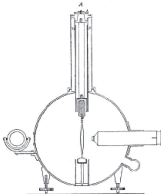
**Fig. 1.1.** The Wulf electroscope.
