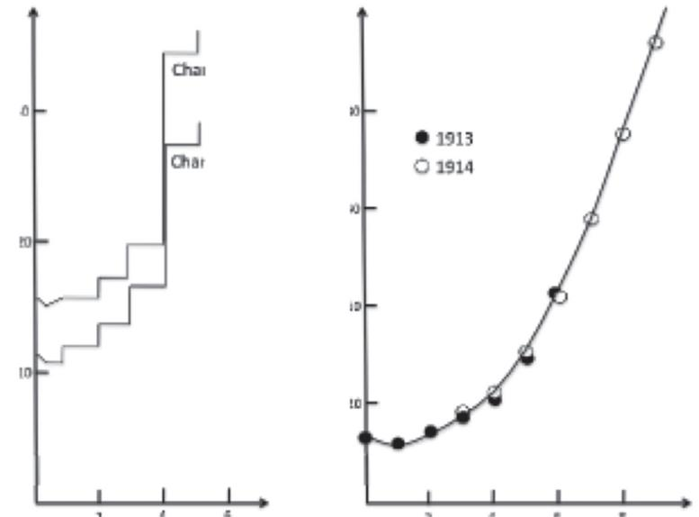
**Fig. 1.4.** Variation of ionization with altitude. Left panel: August 7th's ascent by Hess (1912), where he carried two ion chambers (chamber 2 was shielded with thicker walls). Right panel: Ascents by Kolhörster (1913, 1914).
